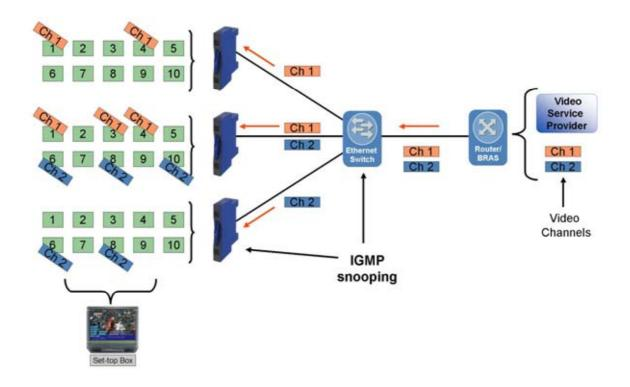
Figure 54 IP Multicasting using IGMP Snooping for Video Services
