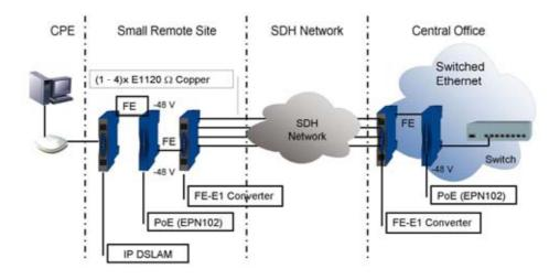
Figure 24 Fast Ethernet to E1 or T1 Converter in a Small Site Solution
