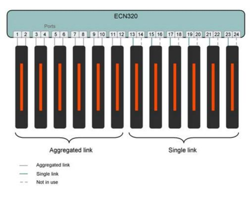
Figure 13 Cabling of Ethernet Cables for Link and PoE Redundancy
