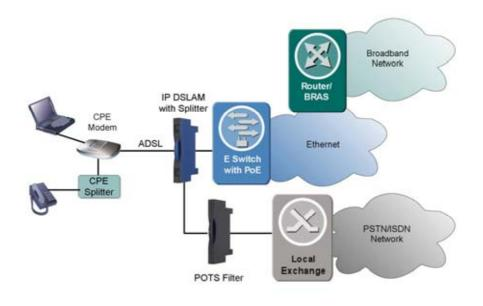
Figure 50 Base band Solution with External POTS Filter
