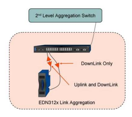
Figure 12 EDN312 Link Aggregation
