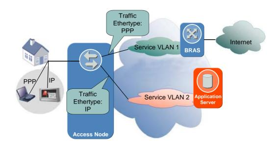
Figure 33 Traffic Mapping to Two VLANs
