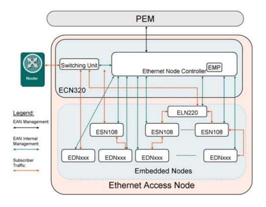
Figure 15 Ethernet Access Node Structure
