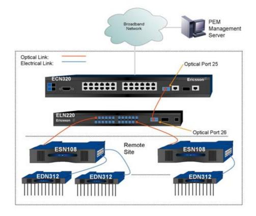
Figure 19 The ELN220 as an Embedded Node in the EAN
