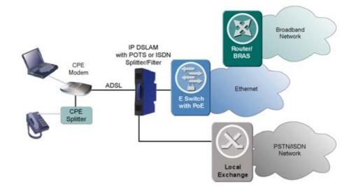
Figure 49 Base band Solution with Integrated POTS/ISDN Filter
