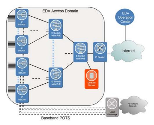
Figure 60 Base band POTS with and without Service Selection
