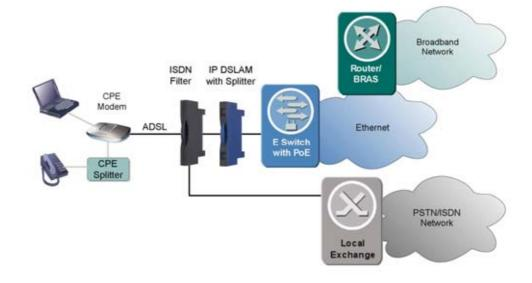
Figure 51 Base band Solution with External ISDN Filter
