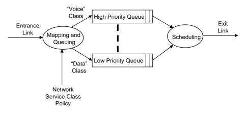
Figure 39 Differentiated Services in an Ethernet Switch
