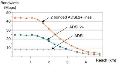
Figure 2 Line Bonding Utilization
