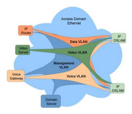
Figure 55 Separation of Traffic Types with VLANs
