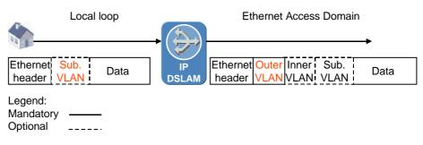
Figure 35 Using QinQ in EDA
