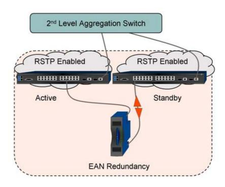
Figure 11 Cabling of Ethernet Cables for EAN Redundancy
