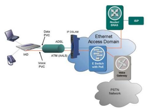
Figure 52 Telephony over IP Architecture
