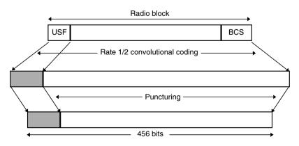
Figure 1.18. Radio block structure for CS-1 to CS-3
