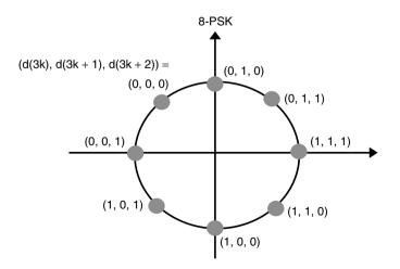
Figure 1.25. 8-PSK signal constellation
