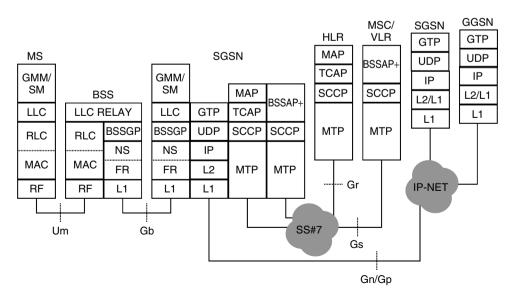
Figure 1.12. GPRS control plane
