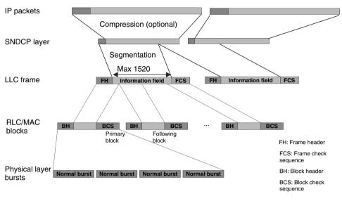
Figure 1.20. Transmission and reception data flow
