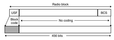
Figure 1.19. Radio block structure for CS-4 [14]
