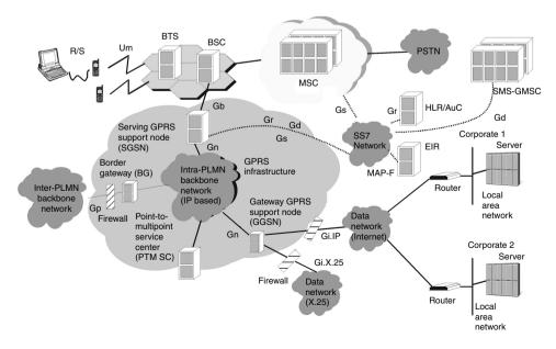
Figure 1.6. Functional view of GPRS
