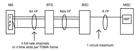
Figure 1.3. Network architecture for supporting HSCSD
