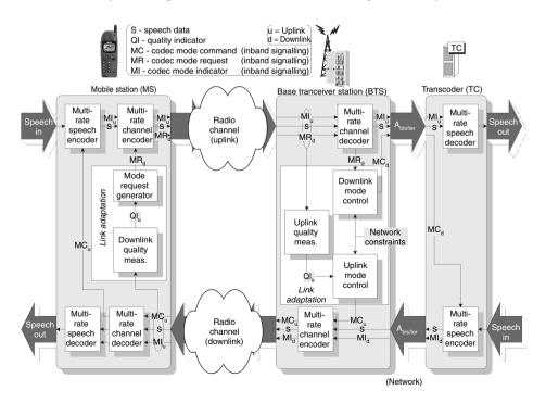
Figure 1.2. Block diagram of the AMR codec system
