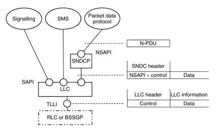
Figure 1.13. Multiplexing of network protocols
