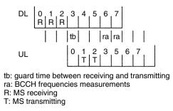
Figure 1.21. Dynamic UL allocation example
