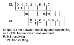
Figure 1.22. Extended dynamic UL allocation example
