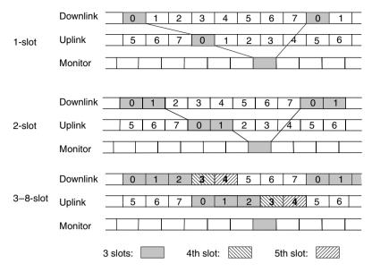
Figure 1.9. GPRS multislot capabilities
