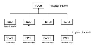
Figure 1.15. GPRS logical channels
